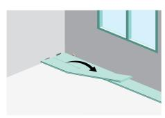
Push to slide the plank against the row in front so it aligns with the first plank. Push it down like with the first plank when the plank is positioned tightly together.
