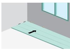
For irregular wall, the plank must be marked as per the outline of the wall and cut accordingly.
