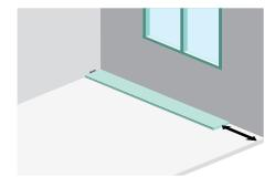
At the end of the first row, leave an expansion gap between 8mm to 15mm against the wall and measure the length of the last plank to fit.
