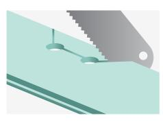
The installation of the heat dissipating pipe is as above image, mark the center of the pipe hole on the plank, then drill holes on the floor with the diameter which is 16mm larger than the diameter of the heat dissipation pipe (for expansion gap of 8mm between plank and the pipe).
